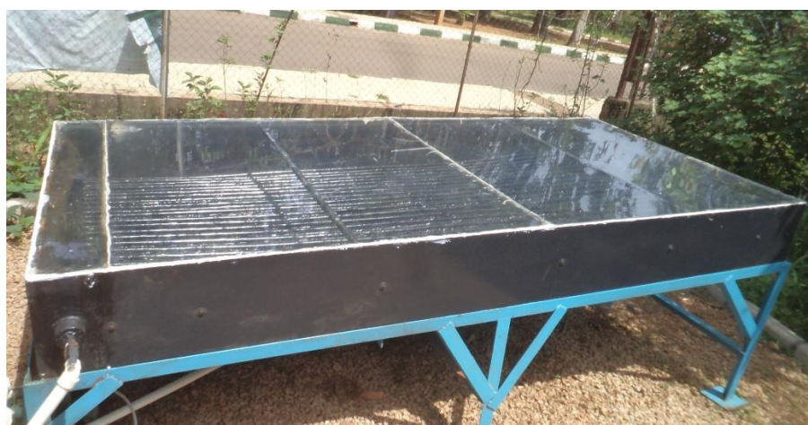
Figure 2b. Pictorial view of Solar Collector after Cover is placed on it
