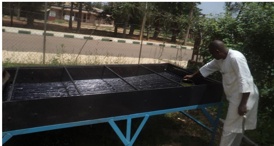
Figure 2a. Pictorial view of Solar Collector before cover is placed on it
